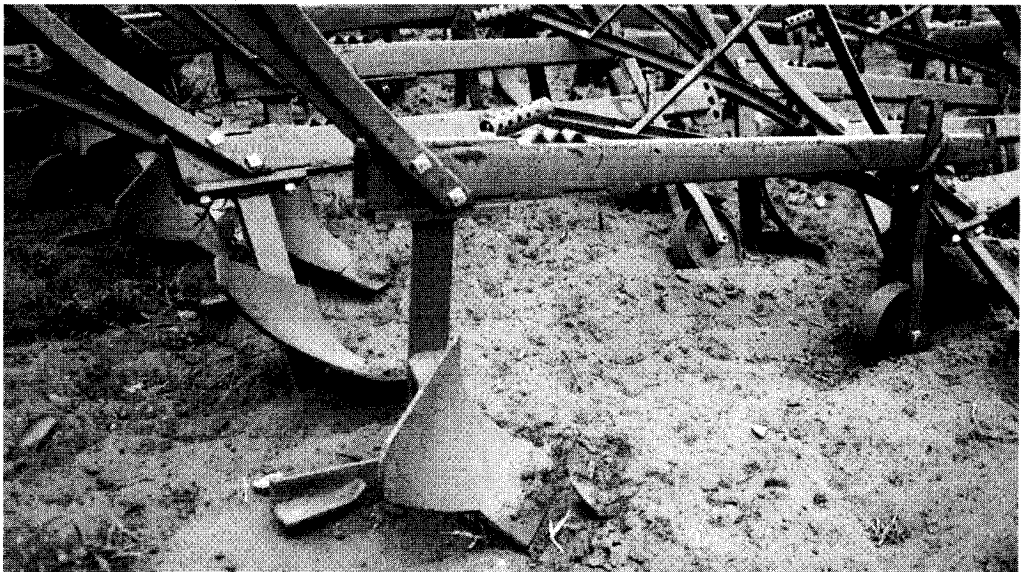
Fig. 11-6: Stockpile of plows imported into Mozambique by a donor-assisted project. The plows have numerous technical defects: for example the mouldboards and shares have no bolts but have been welded in place, making replacement in a small village almost impossible.
