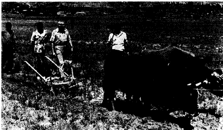
Fig. 7-15: Ariana toolframe fitted with two wheels and a mouldboard plow being used in a "hands-off" plowing demonstration in Lesotho. (The designer of the Ariana , Jean Nolle, is walking beside the plow).
