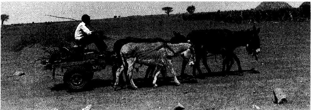
Fig. 8-15: Cart based on old vehicle axle being pulled by team of donkeys in Botswana.
