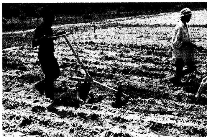
Fig. 9-11: An operator lifts a ridge-tying implement and so forms a ridge-tie. The "Unibar" multipurpose toolbar fitted with the ridge-tier was being tested on a research station in The Gambia.
