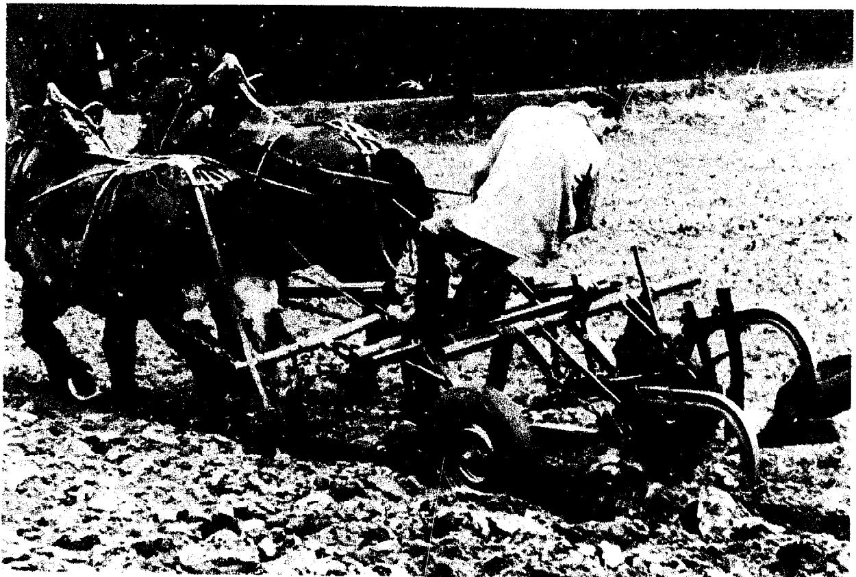
Fig. 2-8: Nolle Hippomobile used as "Sulky" plow in France, 1961. (Photo: Jean Nolle).
