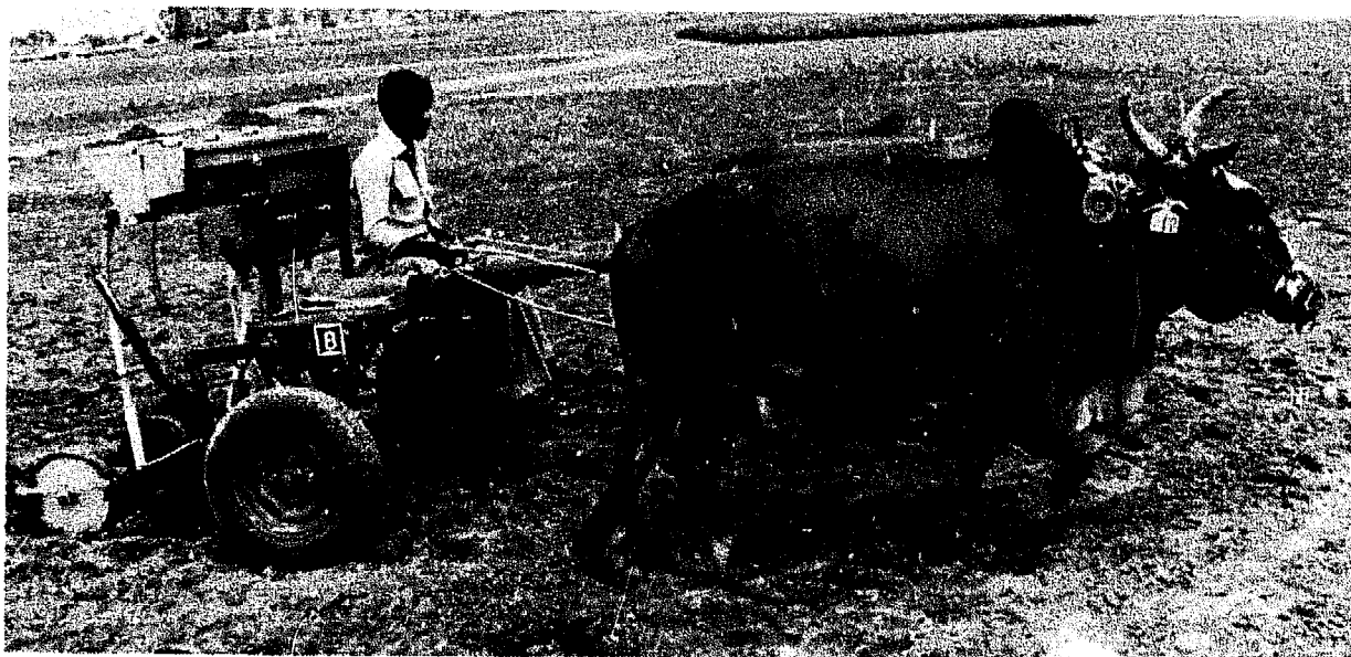
Fig. 2-16: Designed in 1962, modified by ICRISAT, and promoted worldwide, the Tropicultor spans all phases of development. Here seen with seeder and fertilizer distributor at ICRISAT Centre, 1985. (Photo: P.H. Starkey).
